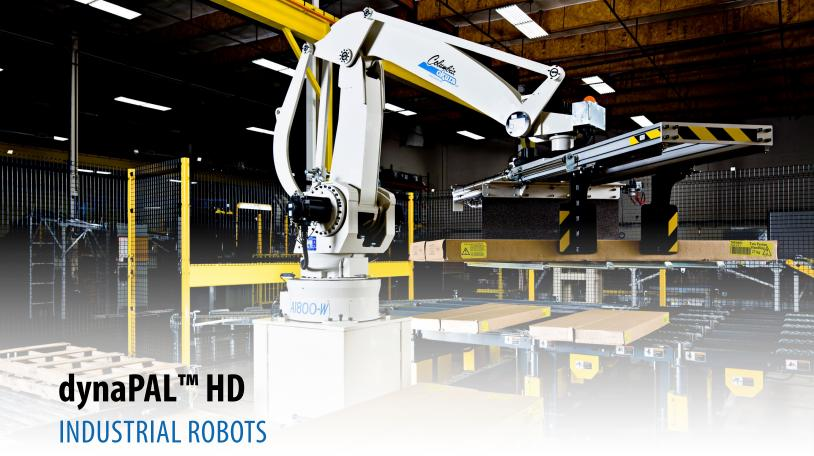
The dynaPAL™ HD is a high-performance palletizer, offering exceptional durability, reliability, and strength. With a payload capacity of up to 350 kg, this robust system handles a wide range of products, including bags, cases, bundles, pails, spot packs, and trays. Designed to excel in demanding environments, the dynaPAL™ HD automates challenging tasks that are often beyond human capabilities.
