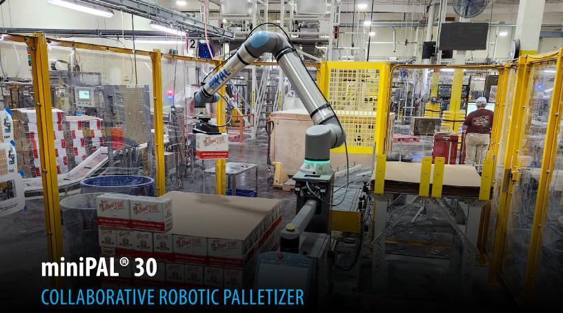
The miniPAL® 30, offering a combined payload of 30 kg (66 lbs) offers a small footprint while still providing a fexible and robust palletizing solution. Containing integrated safety system, the miniPAL® 30 utilizes area scanners, radar and guarding, as well as the built in force limiting technology to offer safety and speed in an optimized footprint.
