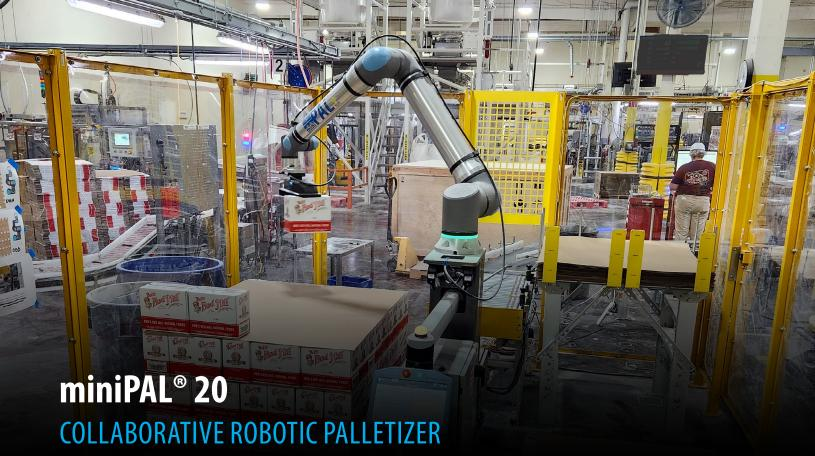
The miniPAL® 20, offering a combined payload of 20 kg (44 lbs) offers a small footprint while still providing a fexible and robust palletizing solution. Containing integrated safety system, the miniPAL® 20 utilizes area scanners, radar and guarding, as well as the built in force limiting technology to offer safety and speed in an optimized footprint.
